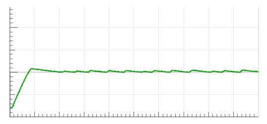
An initial PID implementation based on just the error aims to adjust the power level based on the error.
