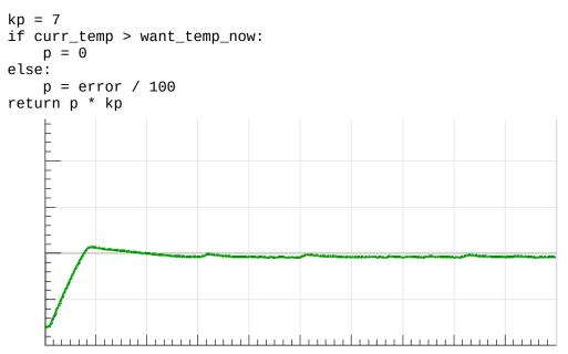
This allows shifting the result around the target temperature, but will require tuning. Observe also that oscillation around the target temperature still occurs. In addition, in digital environments, power levels other than "off" or "on" will require either hardware to permit analogue control, or some sort of dithering algorithm.
